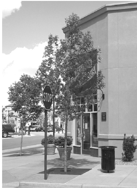
Figure 10 – Utilize human scale design elements such as planters to create a pedestrian friendly entrance to the building.
