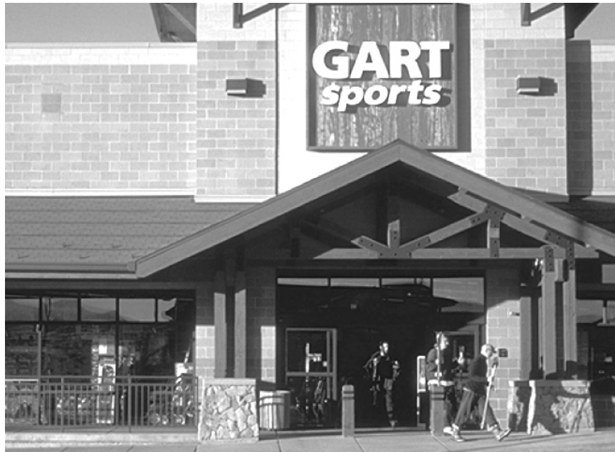
Figure 61 – Use of masonry materials including brick, stone and rusticated block are encouraged.
