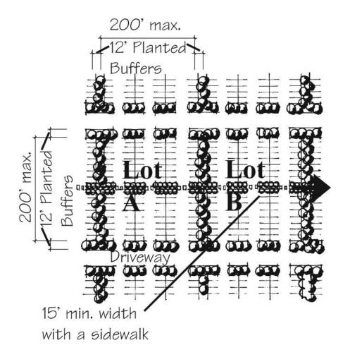
Figure 31 – It is required to divide a large parking area into a series of smaller lots to reduce visual impacts.
