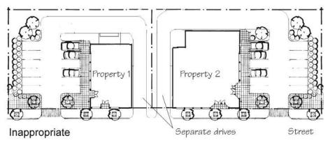
Figure 33 - Eliminate separate or duplicate driveways when feasible.
