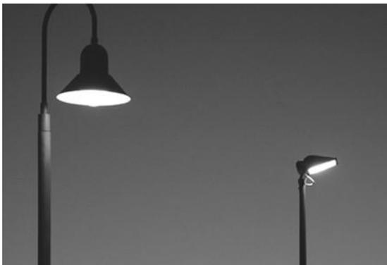
**Figure 35 – All lighting should be directed downward to eliminate light pollution.**
